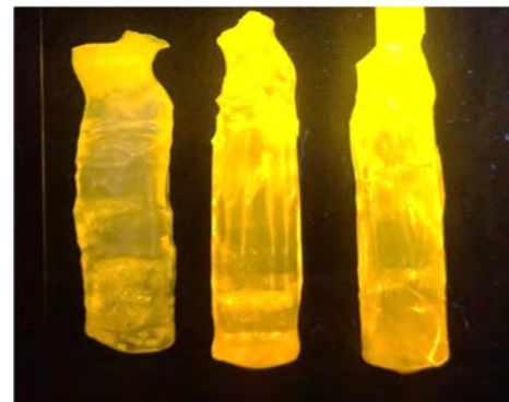
Fig. 1. As grown YAG:Sc,Ce crystals under UV irradiation (Sc content changes from 1 to 25at.% from left to right)
