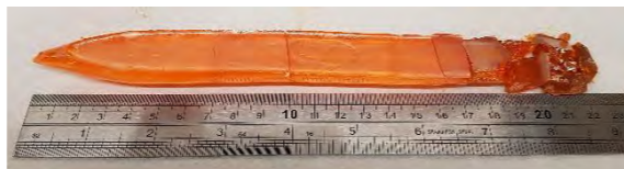
Figure 1: Large single crystal ingot of CsPbBr 3 .
