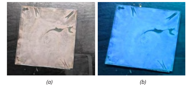
Figure: Cs 3 Cu 2 I 5 :Tl thin film fabricated on flexible substrate (a) under visible light (b) under the UV light
