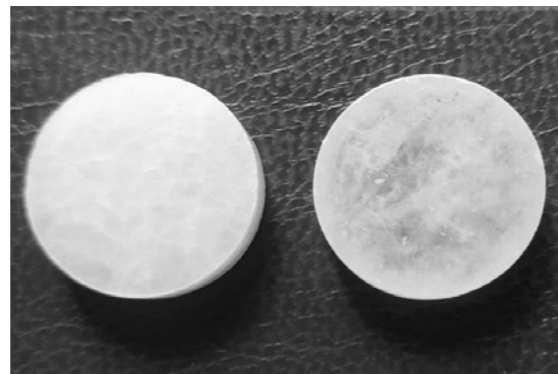
Photographs of p -terphenyl polycrystals with a diameter of d = 20 mm and a thickness of h = 5 mm obtained by hot pressing: (a) a sample obtained by a known method of pressing crystalline granules, (b) a sample obtained by a new method.
