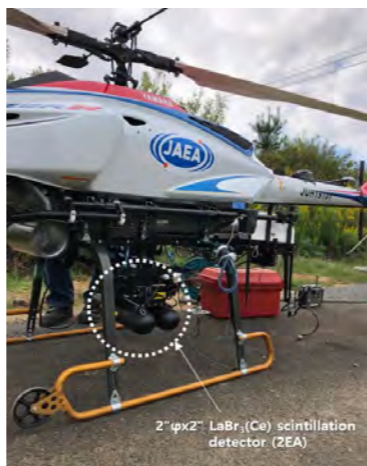
Fig.1. Airborne survey system based on two LaBr 3 (Ce) scintillators of KAERI (UAV: JAEA)
