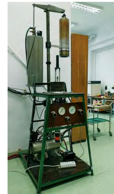
The setup used for the Bridgman growth of Zn x Be 1-x Se crystals.
