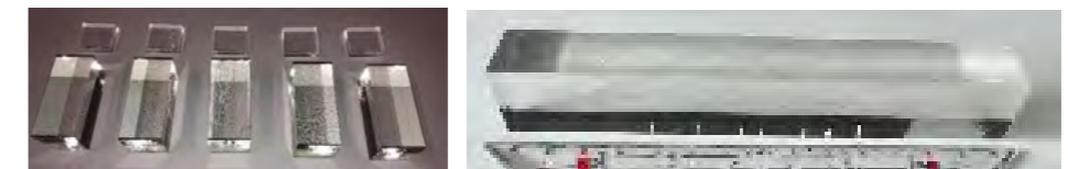
Figure 1. Photos of glass samples delivered by Schott: set of 2 \times 2 \times 0.5 cm 3 , 2 \times 2 \times 5 cm 3 samples (left) and 2 \times 2 \times 15 cm 3 sample (right)
