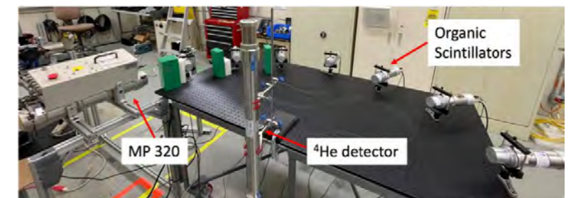
Figure 1: Laboratory configuration for measurement of the 4 He detector response.
