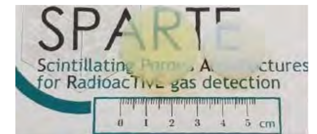
Aerogels before (left, Ce 3+ :YAG, yellow sample) and after (right, Ce 4+ :YAG, white sample) thermal treatment
